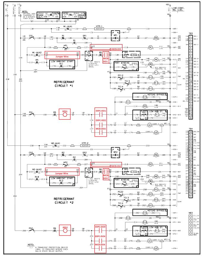
Figure 24: MicroTech I 4-Compressor/8-Stage
