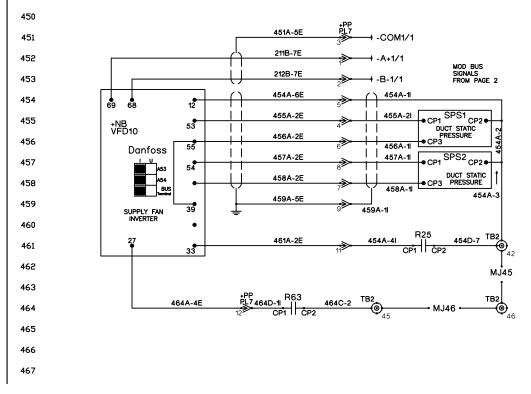
Figure 48: Schneider VFD Wiring
