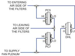
Figure 8: Duct Static Pressure (DSP) Transducer
