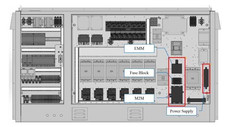
Figure 1: Typical MicroTech Control Panel Layout - 018C - 040C, 800C and 802C
